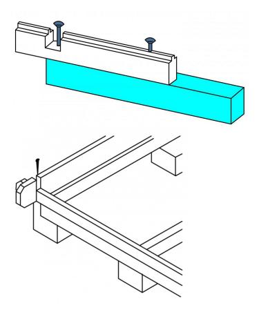
Build up the walls according to the cabin plans. Pay attention to the pre-drilled holes in the wall plank ends and other parts, and make sure you install them strictly to the plan. These hole locations must match the holes of the previous plank rows so that you will be able to insert metal storm braces throughout the entire wall in corners as well as strengthening rods in some wall parts in the later stage.
