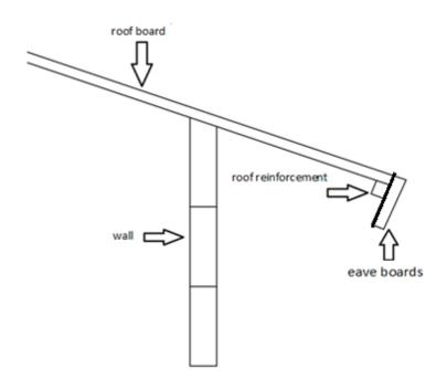
Now mount the roof reinforcement below the eaves, parallel with eave ends. Fix them to roof board by using screws. Then install eave boards to eave ends by fixing them with screws to roof reinforcement. Check that the upper side of the eave board is on the same line and even with the roof.
