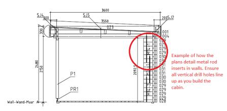
Below is an example of two components the same size but part 009 has vertical drill holes for rods. Be careful not to use the wrong part by mistake.
